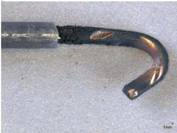
Figure 20. Optical photographs of hot wire removed from receptacle from Circuit 1.
