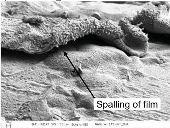
Figure 44. SEM images of the hot wire from the toggle switch in Circuit 3. Note the spalling of the corrosion product film. The contact areas can be seen in the upper two images (bright areas) where the contact shielded the surface from the corrosive gasses.
