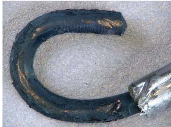
Figure 43. Optical images of the toggle switch in Circuit 3. The figure on the left shows the inside of the switch. Note the extensive corrosion product on some of the components. The image on the right is of the hot wire connected to the toggle switch (screw side).
