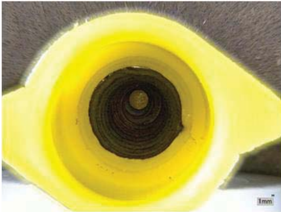
Figure 61. Optical images of twist-on connectors with hot and neutral wires used on the output section of Circuit 2.
