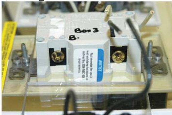
Figure 52. Optical images of the GFCI receptacle. Note the darkening of the normally shiny contact pads and slight corrosion (discoloration) of the screws.
