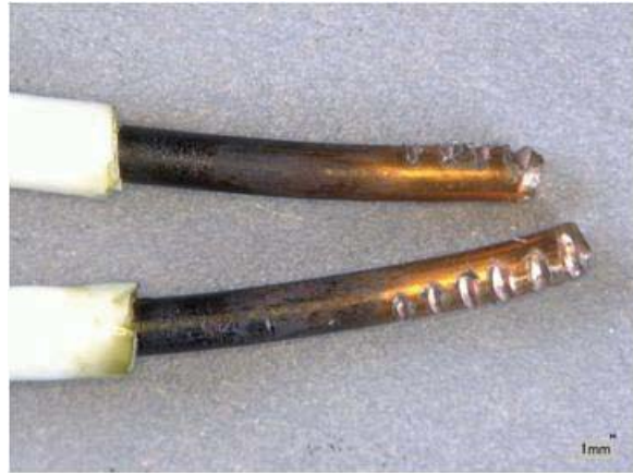
Figure 61. Optical images of twist-on connectors with hot and neutral wires used on the output section of Circuit 2.
