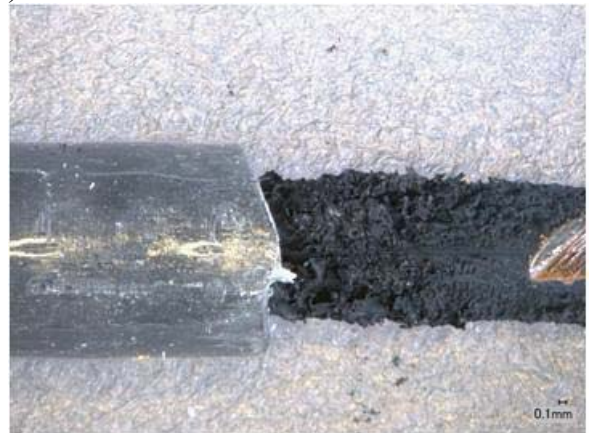
Figure 20. Optical photographs of hot wire removed from receptacle from Circuit 1.
