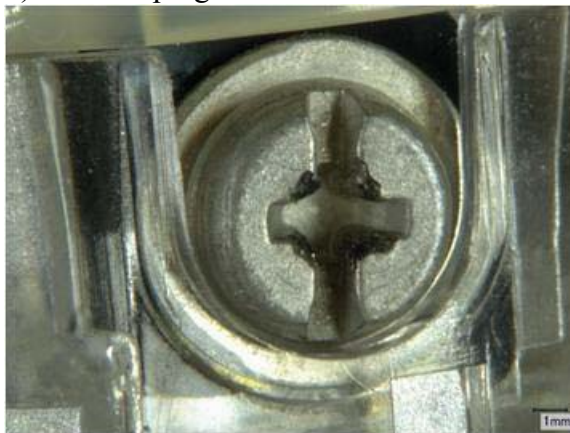
Figure 30. Optical images of the plug used to connect the standard receptacle to the GFCI receptacle in Circuit 1. The prongs and screws are blackened relative to those on a new, as-received, unexposed plug.
