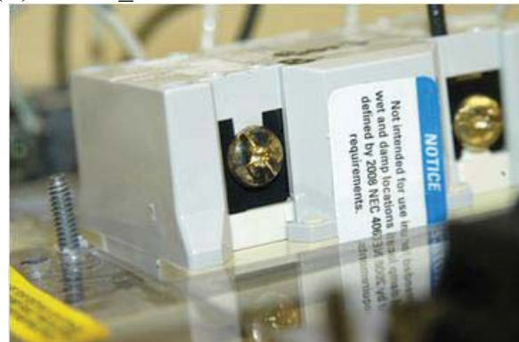
Figure 52. Optical images of the GFCI receptacle. Note the darkening of the normally shiny contact pads and slight corrosion (discoloration) of the screws.
